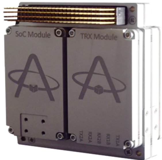
TREVO SDR — SoC and TRX modules
