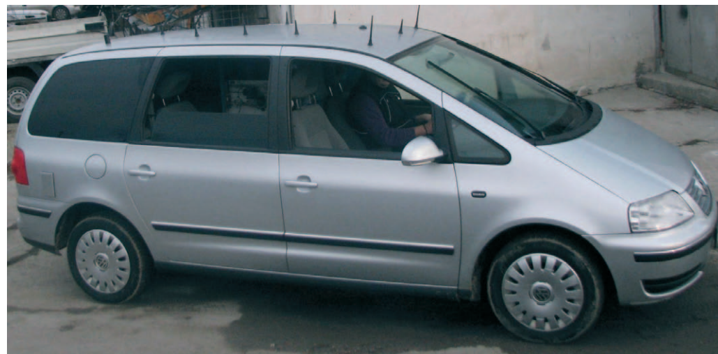
Exhibit 5.11 Special vehicle for measuring level and quality parameters for verification in the mobile communications networks
