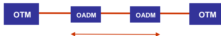
Figure 10 – OTM and OADM in a chain topology and OADM in a ring topology
