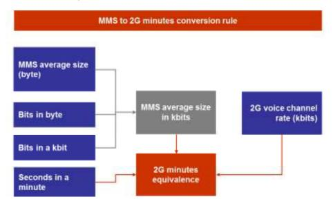
Figure 42 - Data MB to 2G minutes conversion rule
