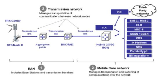
Figure 3 - Scope of the mobile model for illustration purpose
