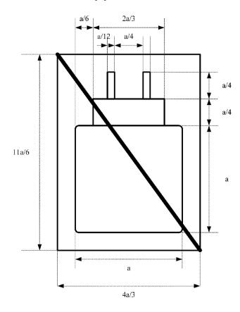
2. The pictogram may vary in appearance (e.g. as to its colour, solid or hollow, line thickness), provided that it remains visible and legible. If the pictogram is reduced or enlarged, the proportions set out in the drawings in point 1 of this Part shall be maintained. The dimension "a" referred to in point 1 of this Part shall be greater than or equal to 7 mm, irrespective of the variation.
